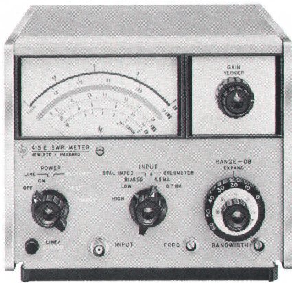
Fig. 2.—hp— Model 415E SWR Meter has scales calibrated in dB and SWR for use with square-law detectors. Instrument has noise figure less than 4 dB when used with common crystal or bolometer detectors. Attenuators are accurate within \pm 0.15 dB.
